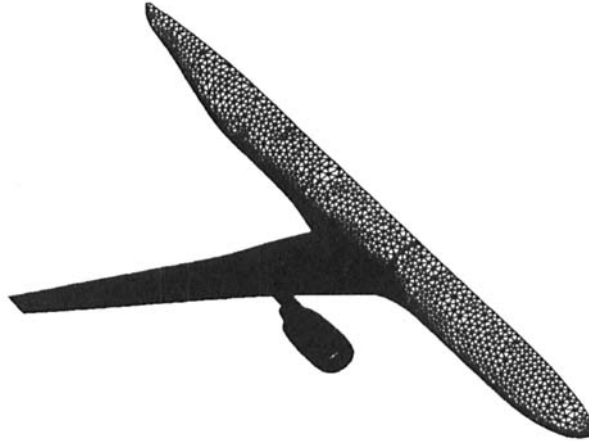
Figure 5. 3D transonic flow past a commercial aeroplane: discretized surface geometry
